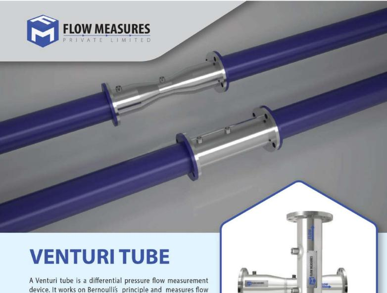
device. It works on Bernoulli's principle and measures flow by detecting the differential pressure created across the throat and the upstream side. Medium entering the venturi through the upstream side is accelerated through a converging nozzle, followed by a diverging diffuser section. Venturi tube is suitable for measuring the flow velocity with minimal pressure drop as the diffuser allows the medium to regain most of its original pressure.
