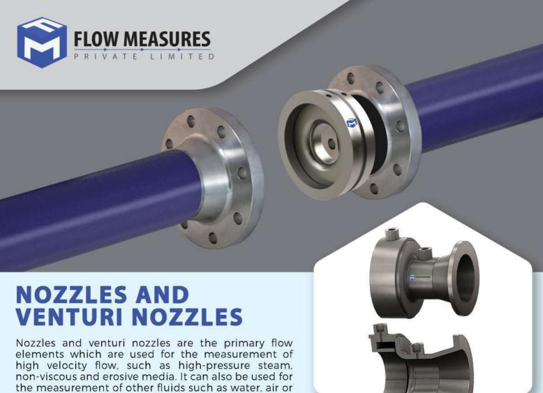
other gases. The design of the nozzles and venturi nozzles are based on Bernoulli's equation and consists of a convergent section with a rounded profile and a cylindrical throat. Due to its rigidity the nozzle is dimensionally more stable at higher temperature and flow rates.
