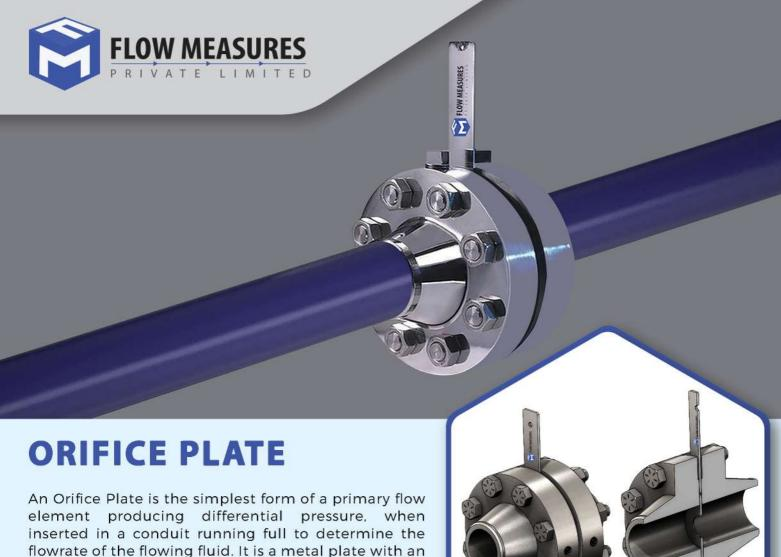
orifice, through which the fluid flows. The differential Pressure generated is directly proportional to the fluid flow rate. Material of construction is guided by the process parameters including temperature, process medium etc, flowing through the pipe. It is one of the most accepted, efficient and versatile methods of measuring flow.
