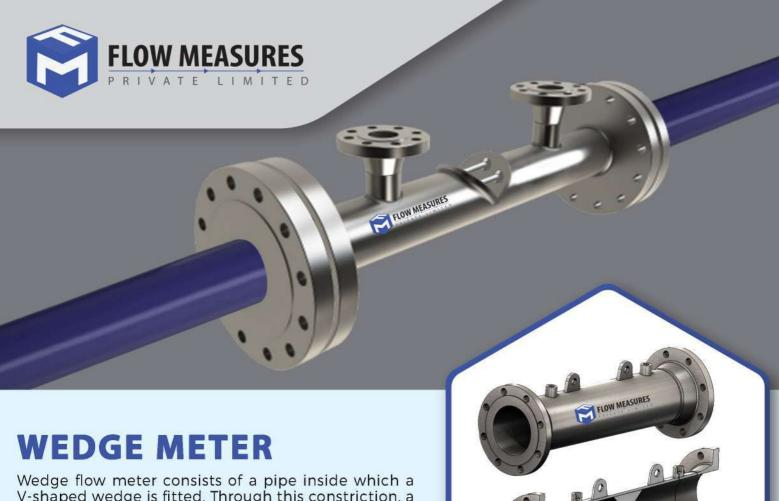
V-shaped wedge is fitted. Through this constriction, a pressure differential is generated proportional to the volume flow rate. Due to the symmetry of the wedge meter, measurement is possible in both directions. The pressure tappings are on either sides of the wedge. Wedge Meter is best suited for the measurement of challenging process fluids such as slurry, liquids with entrained gas, liquids with particles, abrasive fluids etc.
